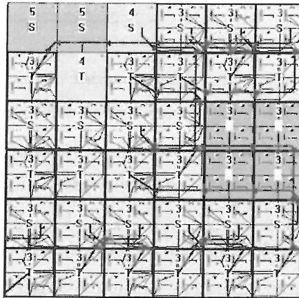
Fig. 13. Screenshot of the growing waveguide string as seen in POETicMol. The string starts on the bottom left. Thick arrows represent cellular connections. Growth takes place by forming forward connections, and cells form backwards connections once they have been activated and the address of their predecessor downloaded. The grey region on the right is intended to simulate a broken cell, which the growth process does not use (connections pass over it but do not end there). The light region at the top left represents the routing process searching for the next active cell.
