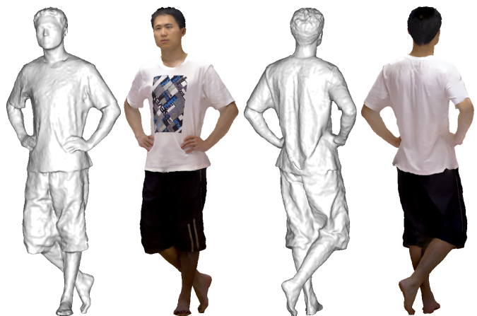
Fig. 1 Two views of a 3D avatar captured using our system, each showing the reconstructed geometry without and with texture.
