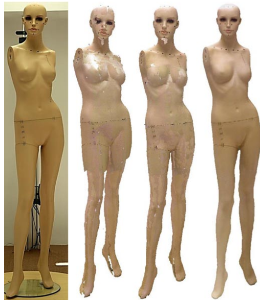
Fig. 4 Calibration with mannequin. Left to right: 2D snapshot from a high-resolution digital camera, 3D coarse alignment from partial scans, alignment after the revised rigid SLAM optimization integrating the color information, and the final textured result.
