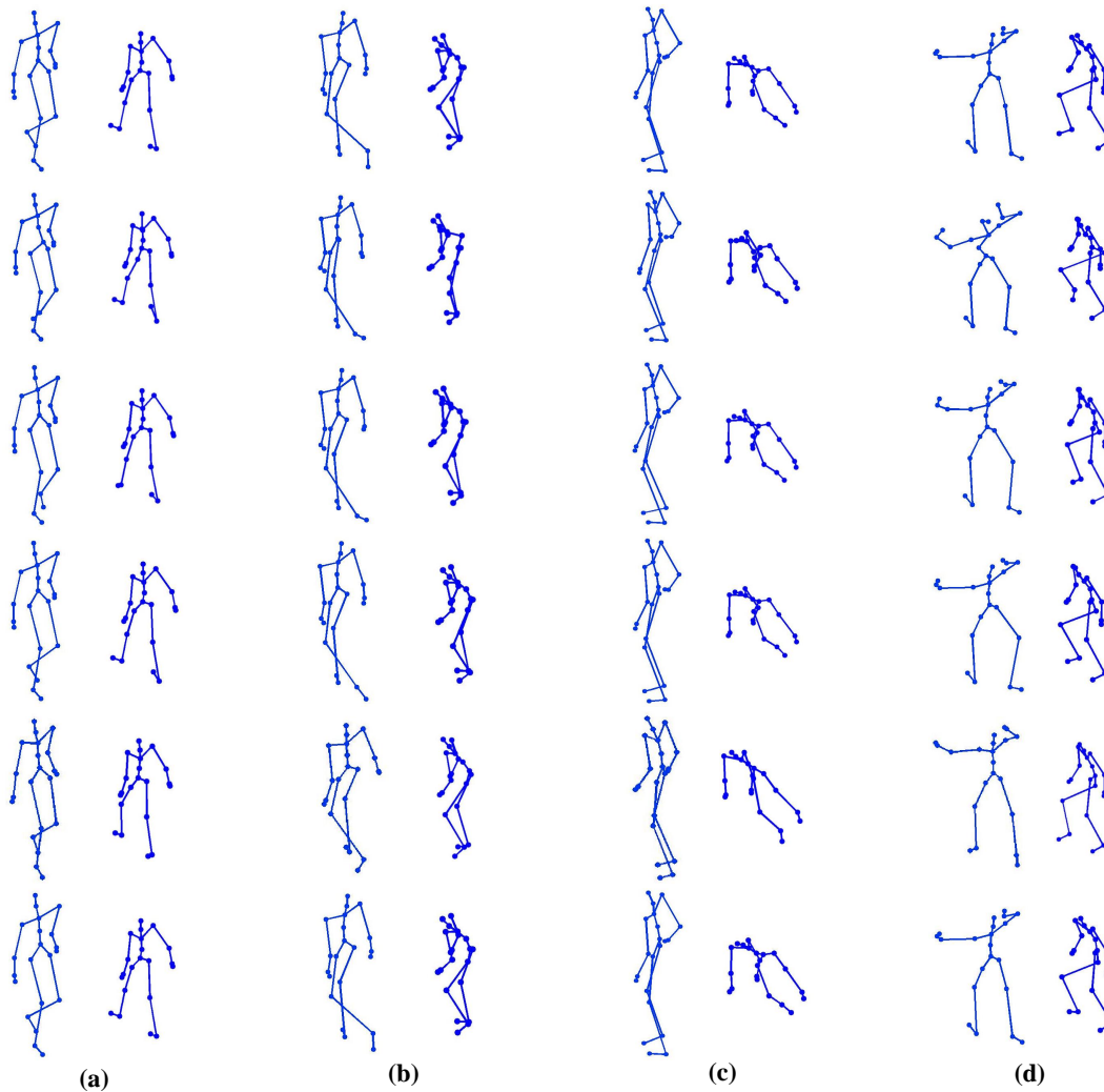
Fig. 8. Comparison results for different sequences of different subjects in the CMU dataset [12] (left in each subfigure) and the Edinburgh dataset [13] [14] (right in each subfigure). From top to bottom: ground-truth skeletons, corrupted skeletons, skeletons recovered by [16], [17], [14], and our method. The corruption rates are: (a) 5%, (b) 10%, (c) 15%, and (d) 20%.
