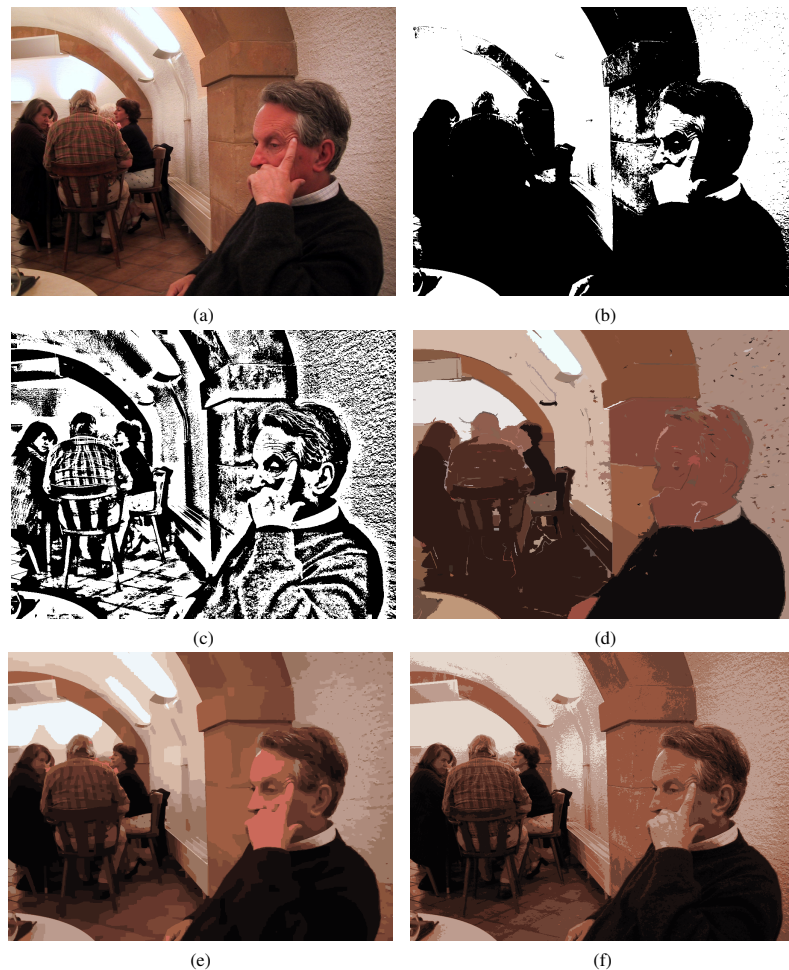
Fig. 11.2 Unsuccessful attempts to render images using computer vision algorithms. (a) source colour image, (b) image with global thresholding, (c) image with local thresholding, (d) segmented image with regions rendered with the mean colour from the corresponding source colour image pixels, (e) alternative segmentation, (f) image with colour quantisation using median cut (10 colours).
