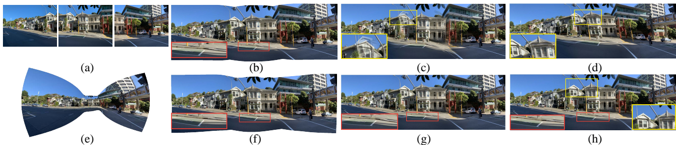
Figure 4. Ablation study of our energy terms for rectangular stitching. (a) input images, (b) initial stitching result, (c, d, f, g) stitching results obtained by removing \phi_a , \phi_s , \phi_r and \phi_l respectively, (e) initial stitching result with a very small weight for \phi_g , as no result is produced without this term, (h) our stitching result using all energy terms.
